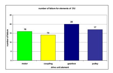
Fig. 17. Number of failures related to elements of drive unit (motor-coupling-gearbox-pulley)
