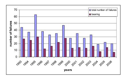
Fig. 14. Failure analysis for pulleys (number of total failures and with respect to bearings)
