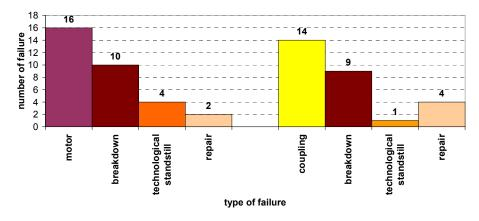
Fig. 20. Number of failures related to DU elements with respect to type of type of event (motor and coupling)
