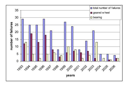
Fig. 9. Number of failures of drive unit gearbox used in CBS
