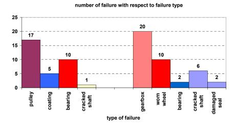
Fig. 19. Number of failures related to DU elements with respect to type of damaged part
