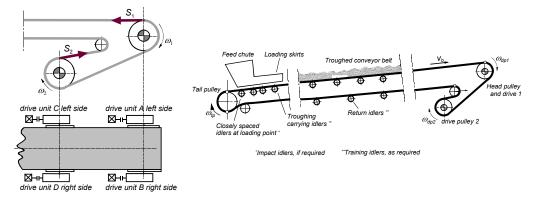
Fig. 3. scheme of belt conveyor [1]
