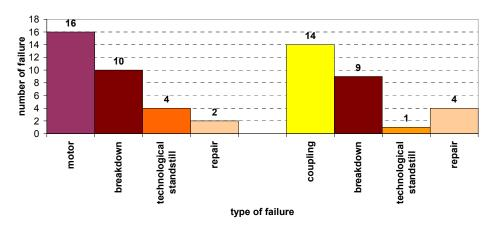
Fig. 21. Number of failures related to DU elements with respect to type of event (gearbox and pulley)
