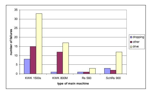
Fig. 13. Number of failures for different types of pulleys used in mine machines in lignite mine
