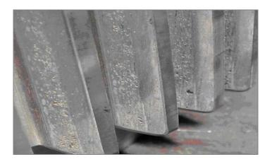
Fig. 11. Example of worn geared wheel
