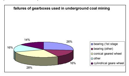
Fig. 10. Percentage of failures for gearboxes used in underground coal mine [6]
