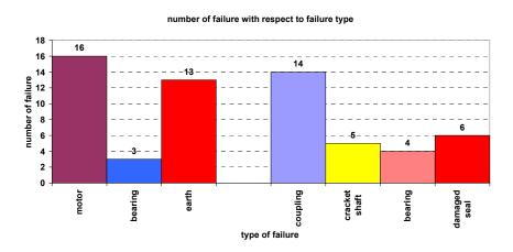
Fig. 18. Number of failures related to DU elements with respect to type of damaged part
