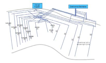
Fig. 1. Scheme of transportation system in the biggest Polish lignite mine [3]
