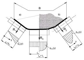
Fig. 22. Distribution of load along belt-idler contact area [9]
